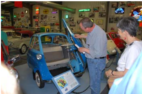
A look inside an Isetta. Notice the steering wheel swings forward to ease entry.
