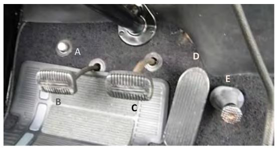
Okay, this month's was a gimme for veteran motorists, but there may be some out there who have never used at least one of these. A: Headlight Dimmer Switch, B: Clutch Pedal, C: Brake Pedal, D: Accelerator Pedal, E: Starter Switch.
