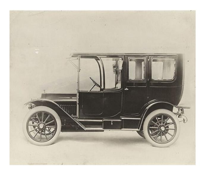
The 1910 Buick Model 41 was the first closed body Buick and first to feature a body by Fisher. The Model 41 boasted a price well above all other Buick models at \$2,750.
